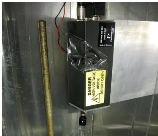
Fig. 24: MP-984-RS Perkin Elmer photon counting module (ICP)
