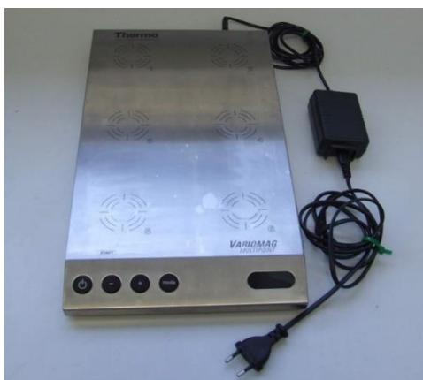
Fig. 25: Variomag Multipoint 6/15 magnetic stirrer (ICP, UTK)
