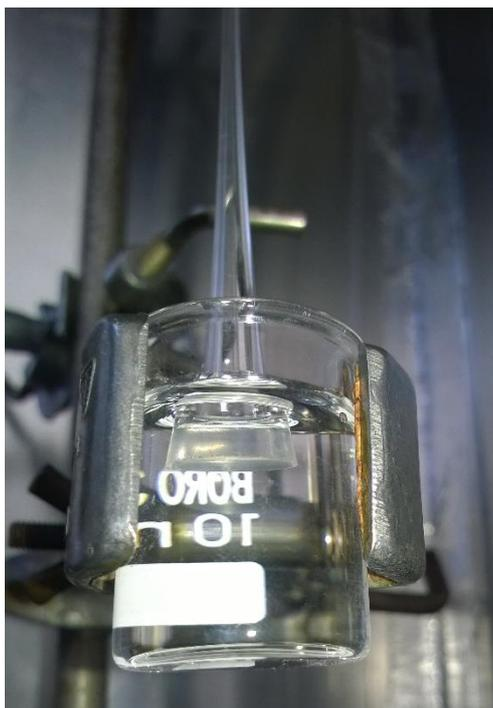
Fig. 38: OFE immersed in the induction solution. Setup was placed in a light-tight box
