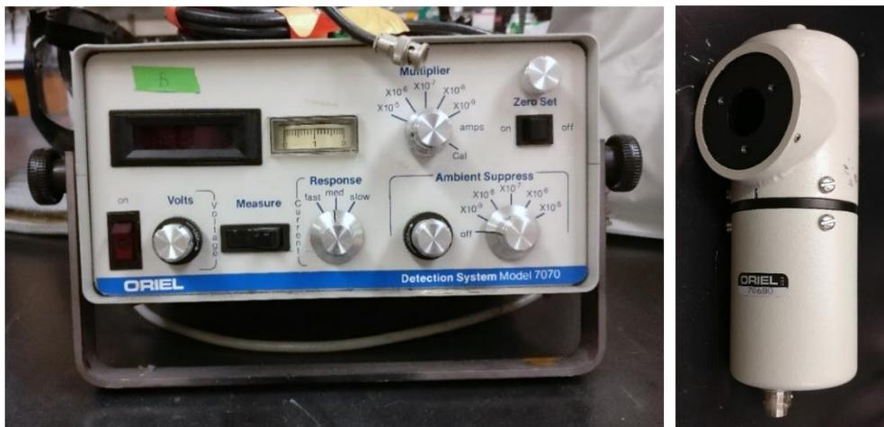
Fig. 23: Oriel 7070 detection system with photomultiplier tube Oriel 70680 (UTK)
