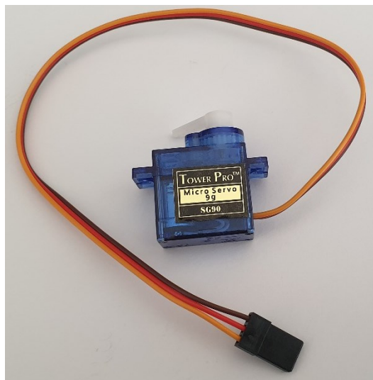
Figure 6: Servo-motor SG90.
