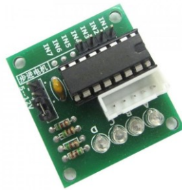
Figure 5: Example of controller circuit for stepper motors. (ULN2003)
