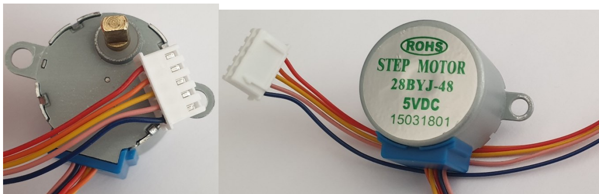
Figure 3: Stepper motor with four coils.
