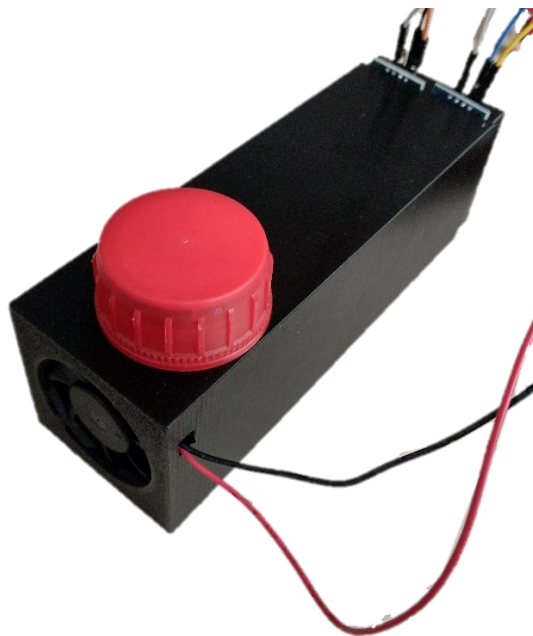
Figure 8: Method of application of the test substance by container cap.
