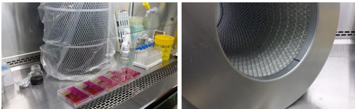
Figure 1 The air filter removed from air conditioning system of Airbus A319 (D. Obitková 2019)
