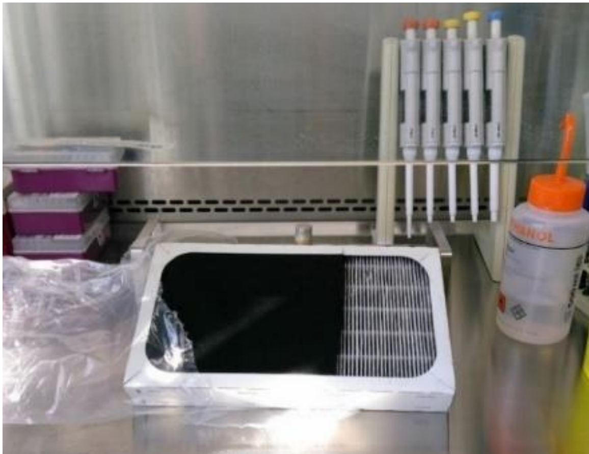
Figure 4 The HEPA filter removed from household air condition (Daniela Obitková, 2019)
