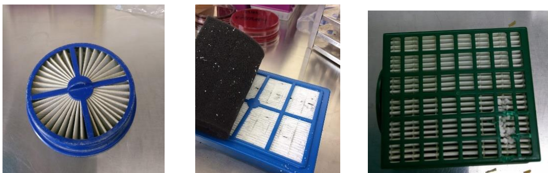
Figure 3 The vacuum cleaner HEPA filters 1, 2 and 3 (Daniela Obitková 2020)
