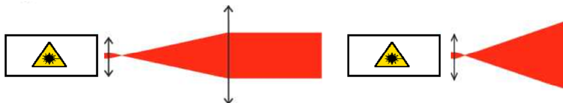
Figure 3: Interferometer arrangement with plane wave (left) and spherical wave (right).
