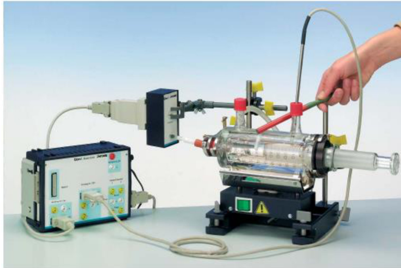
Figure 4. Experiment configuration for Guy-Lussac's and Charles-Amonton's law
