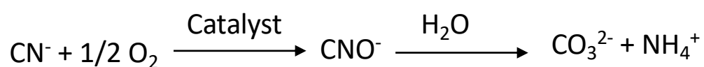
Figure 3. Degradation of free cyanide to the much less toxic cyanate (CNO - ). Hydrolysis of cyanate is optional.
