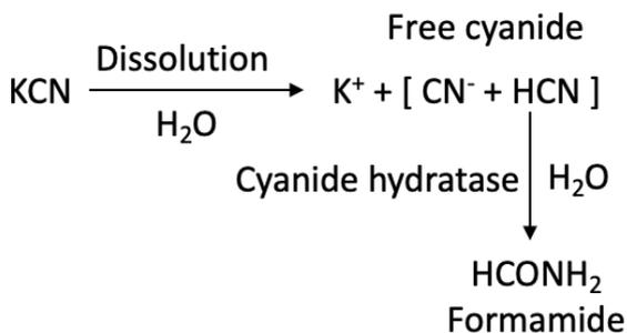
Figure 3. Free cyanide detoxification catalyzed by cyanide hydratases.
