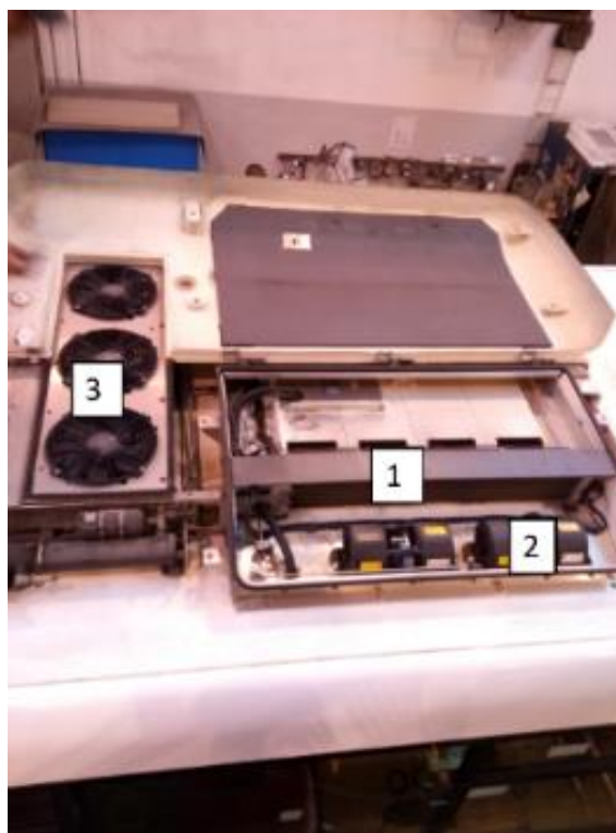
Figure 8 The air conditioning unit on the rooftop of the bus (viewed from the roof of the bus), 1 the evaporator, 2 the ventilator moving the air back to the cabin of the bus, 3 the ventilator removing the undesired heat to the ambient air. (Daniela Obitková 2023)
