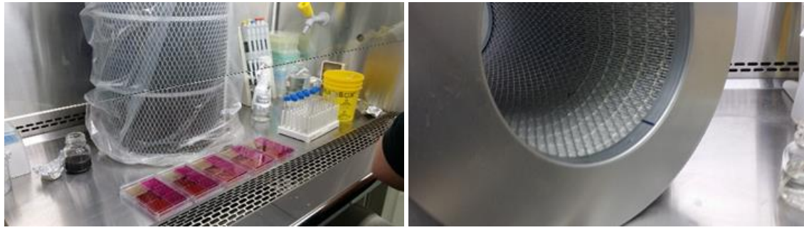
Figure 13 The air filter removed from air conditioning system of Airbus A319 (Daniela Obitková 2019)
