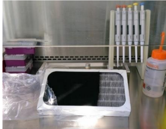
Figure 9 The HEPA filter removed from household air condition (Daniela Obitková 2019)
