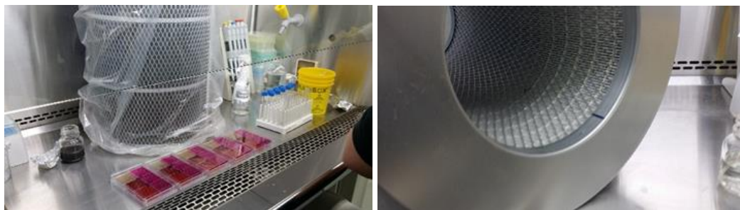
Figure 4 The air filter removed from air conditioning system of Airbus A319 (Daniela Obitková 2019)
